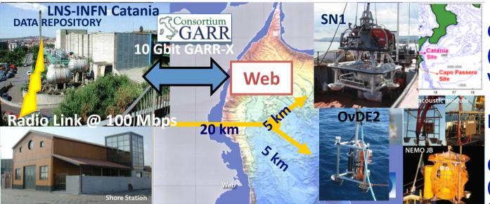
**INFRASTRUCTURE NEMO-SN1 seafloor observatory**, cabled to laboratory in the harbour of Catania by electro-optical cable
